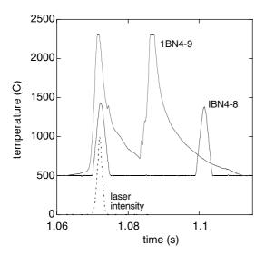
Fig. 2. Temperature response of a deposition region 1BN4-9-z2.1 (upper curve) and erosion region 1BN4-8-4L (lower curve) to two successive passes of the laser spot. The laser time history (measured separately) is shown dotted. The pyrometer operates in the region 500–2300 °C.
