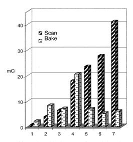
Fig. 3. Tritium released by laser scanning and the subsequent bake in air for samples from JET and TFTR. A variety of scan conditions were used, some not yet optimal. Nonetheless the results illustrate that the detritiation efficiency is high at the locations with the highest concentrations of tritium. The column labels from 1–7 correspond to: JET:IN3-16, JET:1BN4-8, JET:1BN7-15, TFTR:KC22-6E, JET:1BN4-9, TFTR:KC22-6C, JET:PL4B-7 (top).
