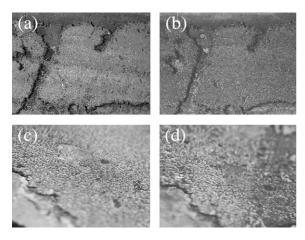
Fig. 5. Images of the tile surface of sample 1BN4-9 before (a) and after (b) two laser scans at 1 m/s, 128 W/mm² in air, peak temperature > 2300 °C; and PL4B7top-6 before (c) and after, (d) three laser scans at 1 m/s, 80 W/mm² in argon, peak temperature 2082 °C. Images (a) and (b) were taken at normal incidence, (c) and (d) at 45°. Each image covers 9.6 mm in the horizontal direction.
