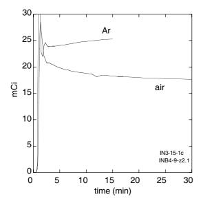
Fig. 4. Tritium concentration vs. time after laser scan in argon atmosphere (IN3-15-1c) and air (INB4-9-z2.1).
